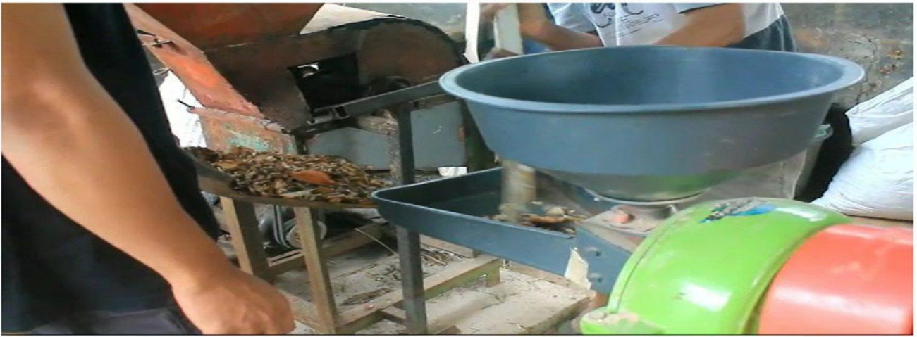
Figure 3. Grinding of dried shells in a disk mill.
